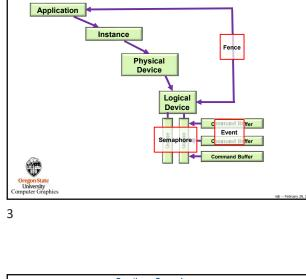
Where Synchronization Fits in the Overall Block Diagram
