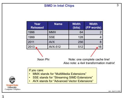
What is Vectorization/SIMD and Why do We Care? 2 Performance! Many hardware architectures today, both CPU and GPU, allow you to perform arithmetic operations on multiple array elements simultaneously. (Thus the label, "Single Instruction Multiple Data".) We care about this because many problems, especially scientific and engineering, can be cast this way. Examples include convolution, Fourier transform, power spectrum, autocorrelation, etc. Signal \* Sine and Cosine values Fourier products
