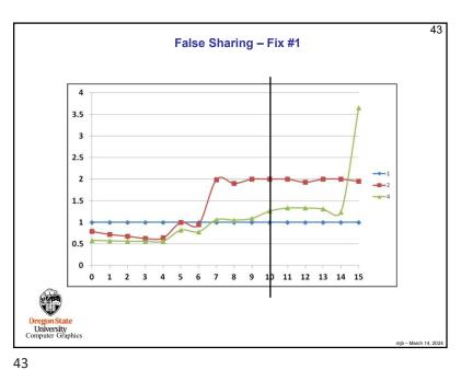
False Sharing – the Effect of Spreading Your Data to Multiple Cache Lines NUMPAD = 10
